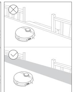
During its first cleaning job, it is recommended to follow the robot to find some possible problems. The robot can clean much more smoothly after that. If certain area do not need to be cleaned, you can add No-Go Zones or Virtual Walls on the map via the app to prevent the robot from entering the specified area.
