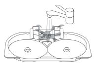
4. Reassemble the left and right cleaning discs and self-cleaning assembly back into the cleaning tray in turn, and then reinstall them at the bottom of base station after drying.
