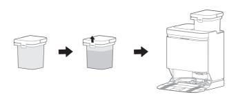
2. To empty the dirty water, remove the Waste water tank on the left, open the cover, and pour out the water.
