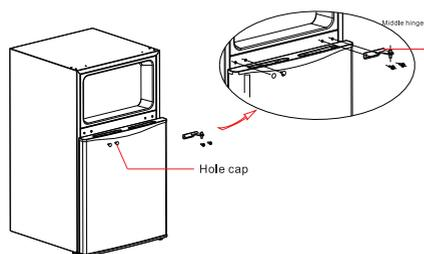
4) Remove refrigerating chamber door and dismantle bottom hinge and adjustable foot.
