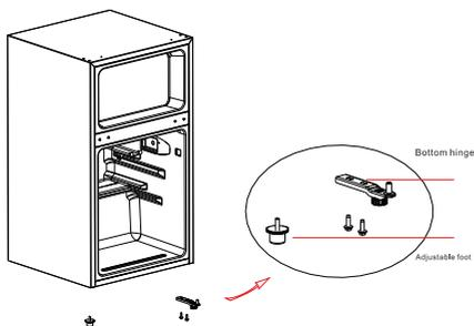
5) Exchange the installation position of bottom hinge and adjustable foot, then fix them respectively. Remove the hinge sleeve pipe of the refrigerating chamber door, and install it on the other side. Remove the hinge sleeve pipe of the freezing chamber door and install it on the other side.
