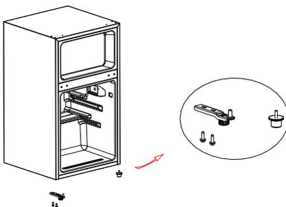
6) Place refrigerating chamber door on bottom hinge, then fix the middle hinge on left side and insert the hole caps on right side.
