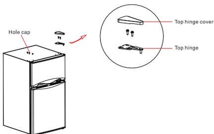
3) Remove freezer chamber door as well as middle hinge and hole cap of the other side.
