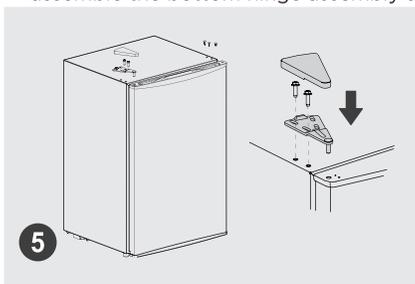
5. Dismantle the stopper under the door then assemble the stopper on the other side. Put the door on bottom hinge and assemble the upper hinge, upper hinge cover and plastic screw hole caps successively.
