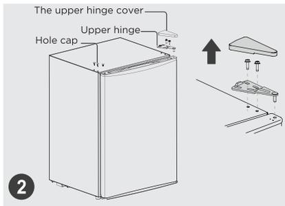
3. Dismantle the upper hinge cover, screws and upper hinge, and remove the plastic screw hole caps from the other side.
