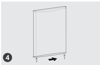
4. Dismantle the door and the bottom hinge assembly and adjustable foot, then assemble the bottom hinge assembly and adjustable foot on other side.
