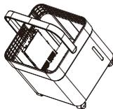
Method B: Remove the rubber plug at the bottom of the bucket to drain off the water.
