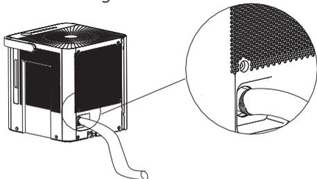
3. The overall height of the tube should be lower than the drain to avoid water backflow and ensure smooth discharge.
