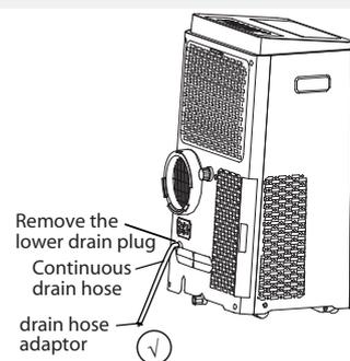
NOTE: Make sure the hose is secure so there are no leaks. Direct the hose toward the drain, making sure that there are no kinks that will stop the water flowing. Place the end of the hose into the drain and make sure the end of the hose is down to let the water flow smoothly. When the continuous drain hose is not used, ensure that the drain plug and knob are installed firmly to prevent leakage.
