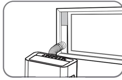
5. Insert the window slider adaptor into the hole of the window slider.
