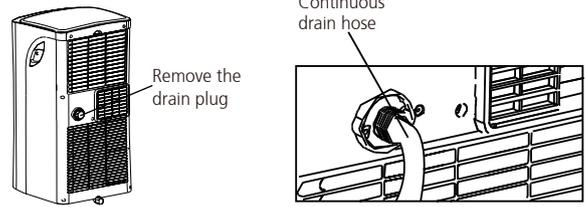
**NOTE:** Make sure the hose is secure so there are no leaks. Direct the hose toward the drain, making sure that there are no kinks that will stop the water flowing. Place the end of the hose into the drain and make sure the end of the hose is down to let the water flow smoothly. When the continuous drain hose is not used, ensure that the drain plug and knob are installed firmly to prevent leakage.
