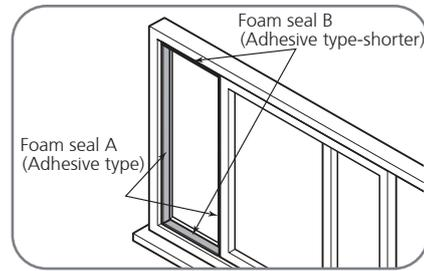
1. Cut the adhesive foam seal A and B strips to the proper lengths, and attach them to the window sash and frame as shown.
