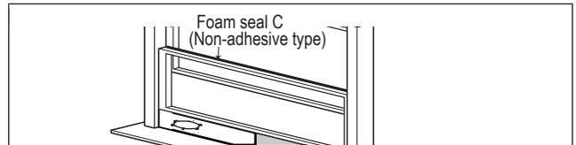
Cut the non-adhesive foam seal C strip to match the width of the window. Insert the seal between the glass and the window frame to prevent air and insects from getting into the room.
