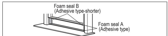
Cut the adhesive foam seal A and B strips to the proper lengths, and attach them to the window sash and frame as shown.
