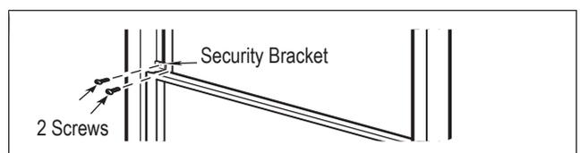
If desired, install the security bracket with 2 screws as shown.
