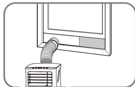
Insert the window slider adaptor into the hole of the window slider.
