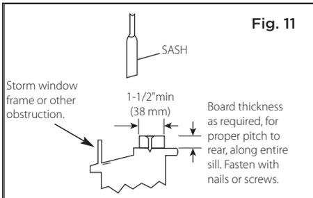
Add wood as shown in Fig. 11, or remove storm window before air conditioner is installed.
