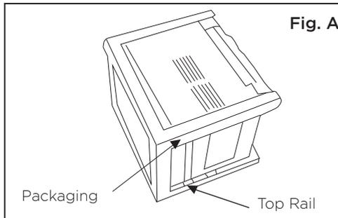
A: Remove the air conditioner from the carton and place on a flat surface.
