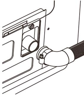
3. Move the clamp toward the drain pipe outlet. Tighten the clamp with a flat blade screwdriver.
