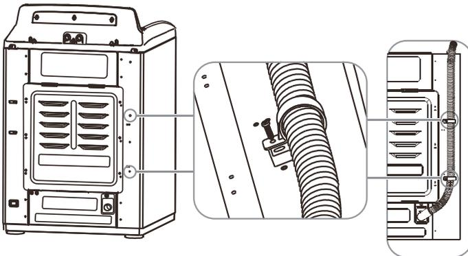
5. Insert the drain hose with the clamp onto the washer's drain pipe. Make sure that the drain hose completely covers the end of the drain pipe.
