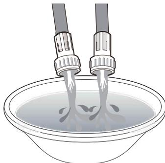
4. Connect the ends of the water supply hoses to the water supply intake connections at the top of the washer. Make sure that the rubber washers are in place. The water supply hose connected to the hot faucet must be connected to the hot water supply intake and the water hose connected to the cold faucet must be connected to the cold water supply intake.
