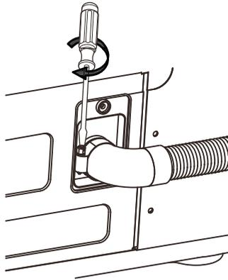
4. Fasten the drain hose to the washer frame at the indicated directions with the hose clamps (2) provided, using a phillips screwdriver.
