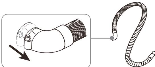
2. Insert the drain hose with the clamp onto the washer's drain pipe. Make sure that the drain hose completely covers the end of the drain pipe.
