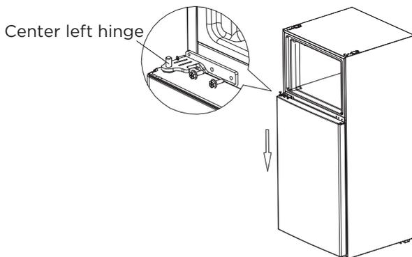
10. Install the freezer door vertically onto the center hinge. Take out the left top hinge and left top hinge cover from accessory bag, assemble left top hinge, left top hinge cover and hole cover.
