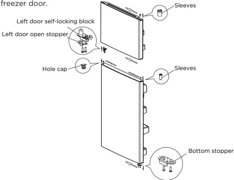
9. Install the refrigerator door vertically onto the bottom hinge. Take out the center left hinge from the accessory bag then assemble the center left hinge on the left side of the refrigerator.
