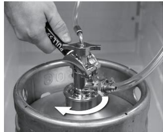
3. Make sure the Tap Tower Is In The Closed (Handle Pointing Straight Up) Position. secure The Connection By Pulling The Coupler Handle Out And Pushing Down Until It Locks Into Position. The Pull Handle Will “Click” When It Shifts Into The Final Downward Position. This Will Open The Beer And CO<sub>2</sub> Gas Valves. The Keg Is Now Tapped.
