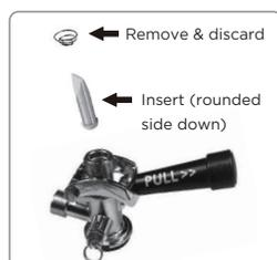
Remove the black packing cap from the top of the Coupler, then place the Top Coupler Washer flush and centred on the top of the Keg Coupler.
