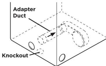
3. Insert the 4 inches (10.2cm) elbow through the rear opening and attach it onto the adapter duct.
