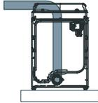
Clean all old ducts before installing your new dryer. Be sure the vent flap opens and closes freely. Inspect and clean the exhaust system annually.
