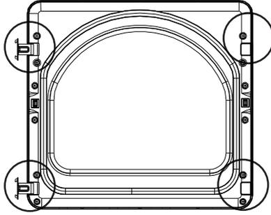
2. Use a flat-head screwdriver to pry open the 5 tabs, pull the inside door panel from the outside door panel.
