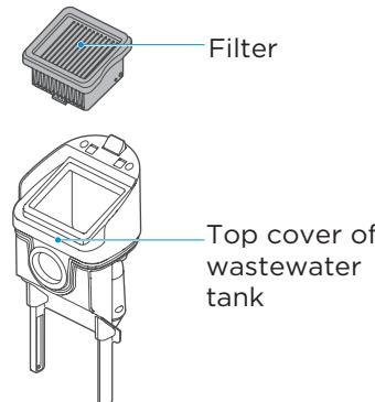
5. Wash with clean water after removal, thoroughly dry it, and put it back in its original position.
