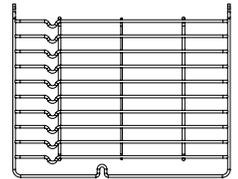
Telescopic runner: Some models might with telescopic runners to facilitate the use of oven. These telescopic runners and slider brackets could be disassembled by unscrewing the screws used to fix it. After disassembled, dishes and tray can be put on the oven floor, using functions as Radiant grilling, Double grilling, Double grill with fan.
