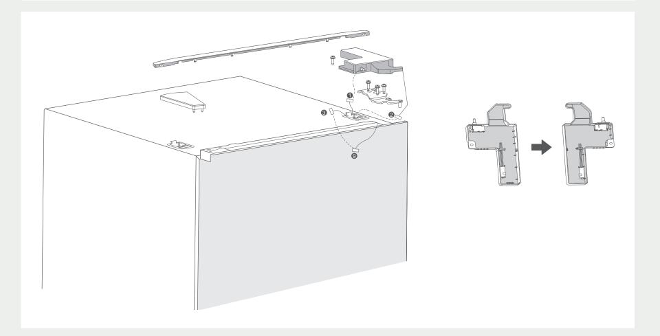
3. Remove the refrigeration door body (pay attention not to lose small parts such as door stoppers);
