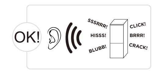
**CLICK:** Some electrical parts in the refrigerator, such as electric valve will make this noise when working. This is normal.
