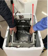
17. Undo the Magnetic Cover Switch
