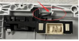
6. Undo the Water Level Sensor
