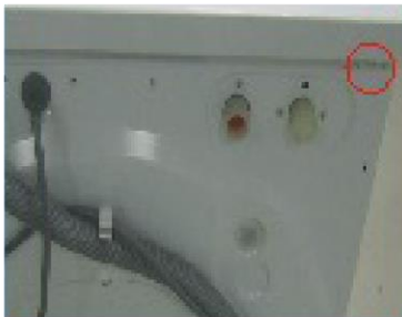
Fig.4 Undo the top cover
