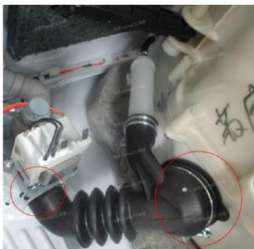
Fig.8 Remove the connection between the black pipe and the tub, remove the connection between the black pipe and the pump
