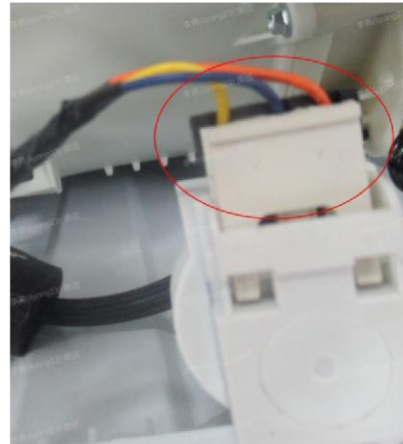
Fig.11 Remove the terminal of the water level sensor
