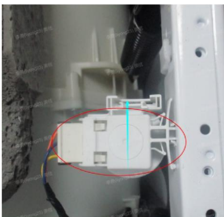
Fig.12 Rotating the sensor to remove the water level sensor from the box
