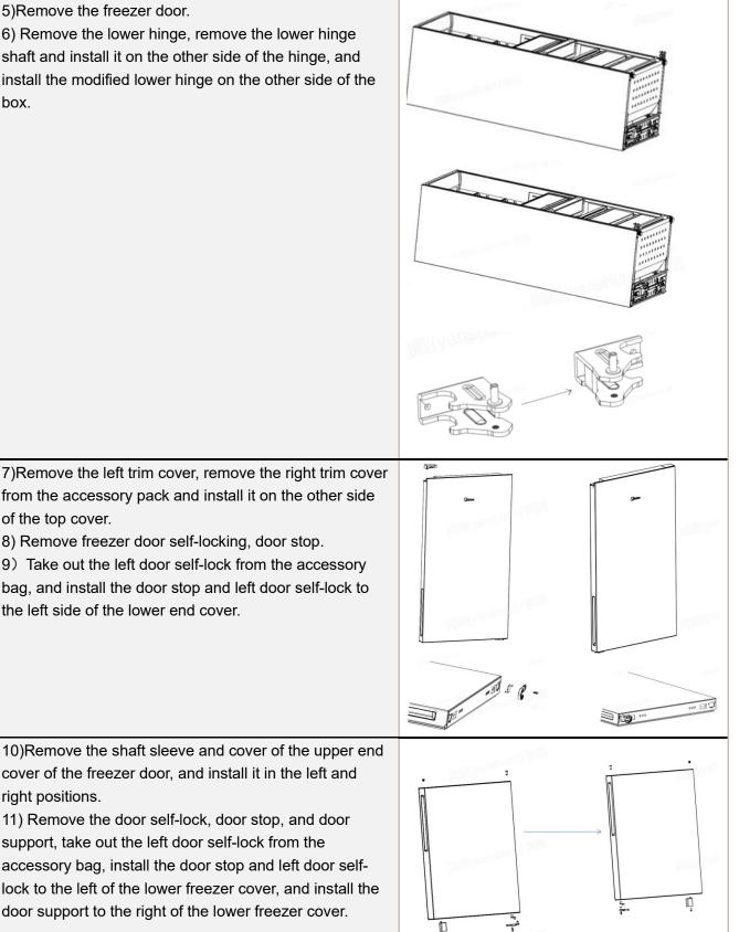
7)Remove the left trim cover, remove the right trim cover from the accessory pack and install it on the other side of the top cover.
