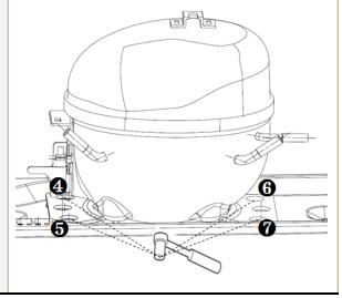
8) Use Pipe cutter cut off the condenser tube (3), then Shear off capillary **9** by the capillary tube scissors. 9) Replace the compressor and welding the compressor pipeline. -10 Welding the process pipeline. -**11**Welding the low-pressure muffler. - Welding the high-pressure exhaust pipe. 10) Replace the filter, Cu-Fe tubes welding **(B)** used Ag welding rod, Cu-Cu tubes welding used Cu welding rod. 11) Vacuum system, The degree of vacuum below 6Pa. 12) Perfusion refrigerant.
