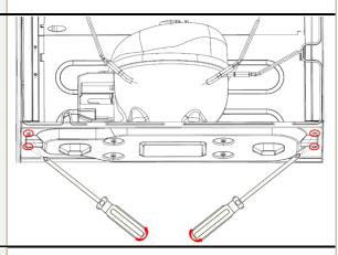
7) Use the wrench to remove the bolts by steps **466 7**, replace the compressor and reverse process can complete installation.
