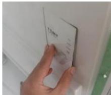
The display panel uses two screws to secure the display panel. Remove the screws and take out the display panel
