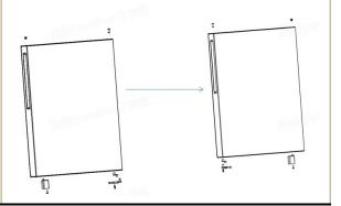
12)Install the reassembled freezer door on the lower hinge, then install the middle hinge, and cover the hinge hole decoration cover
