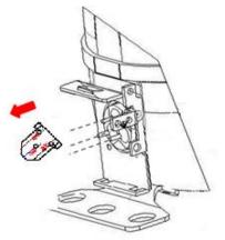
6) Loosen the screw of the compressor bottom plate, remove the floor together with the compressor from the box.
