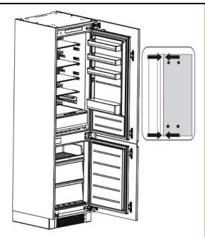
5) Take out the sealing strip from accessory bag, and press it in the gap between the cabinet and the refrigerator. Installation is completed.
