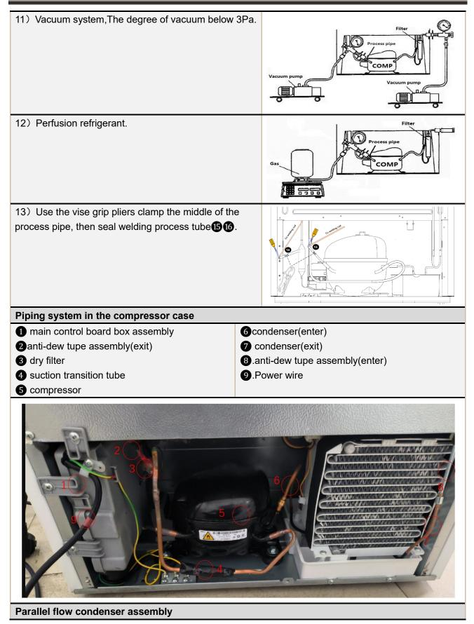
Remove the fixing screws of the side water tray, 1) unplug the fan terminals and drainage pipes, cut off the pipes, and manually remove the entire parallel flow component for replacement 2) Replace the parallel flow condenser assembly, the reverse process can complete installation.
