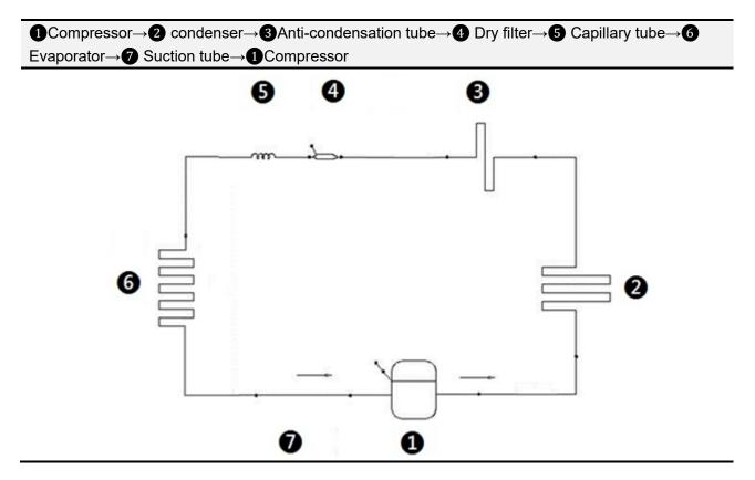
6.2 Cooling pipeline and drain pipe inside the cabinet
