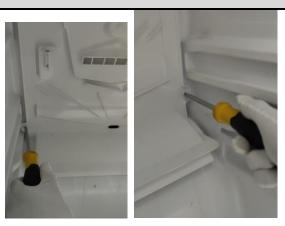
2) Pull out the connector terminal of the fan motor llin 1111 and the sensor. IN IN Fan Remove the aluminum foil and sponge from the 1) rear panel of the air duct, and then manually remove the rear panel of the air duct outward to expose the fan. The fan is fastened with three screws, removing 2) screws and removed 1111
