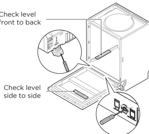
**⚠** The maximum adjustment height of the feet is 50 mm.
