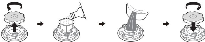
1. Remove the lower basket and unscrew the reservoir cap.
