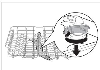
2. To remove the lower spray arm, pull out the spray arm upward.
