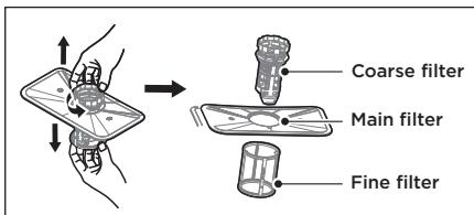
3. Larger food remnants can be cleaned by rinsing the filter under running water. For a more thorough clean, use a soft cleaning brush.
