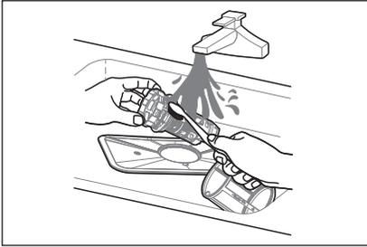
4. Reassemble the filters in the reverse order of the disassembly, replace the filter insert, and rotate clockwise to the close arrow.
