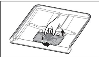
2. The fine filter can be pulled off the bottom of the filter assembly. The coarse filter can be detached from the main filter by gently squeezing the tabs at the top and pulling it away.
