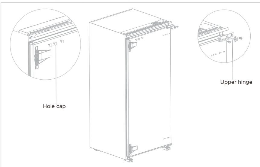
3. Remove the refrigerator door, the bottom hinge and the hole caps.
