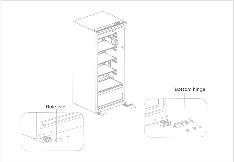
4. Exchange the bottom hinge and upper hinge, then install them according to below steps, and install the hole caps.
