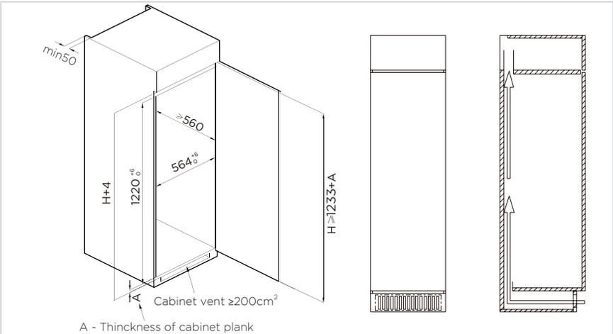
2. Push the refrigerator into the cabinet and adjust it to make sure the edge fold of top baffle completely touch the top edge of the cabinet, and the limit hook of supporting leg completely touch the bottom edge of the cabinet.
