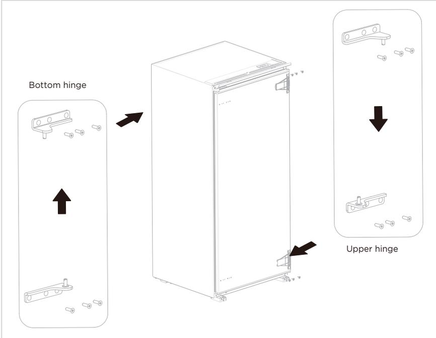
5. Remove the two fixed blocks of refrigerator door and rotate them for 180°, and install them on other side of refrigerator door.
