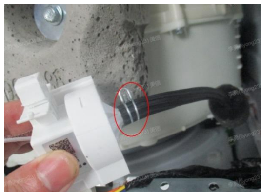
Fig.9 Remove the connection between the black pipe and the water level sensor
