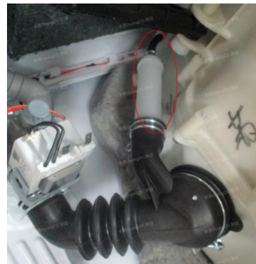
Fig.7 Whether the air pipe is damaged
