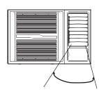
When the AUTO SWING switch is turned to "ON" position, the vertical louvers automatically oscillate right and left sweeping the cold air alternately to obtain comfortable cooling. The vertical louvers may be stopped at any position when the AUTO SWING switch is turned "OFF".
