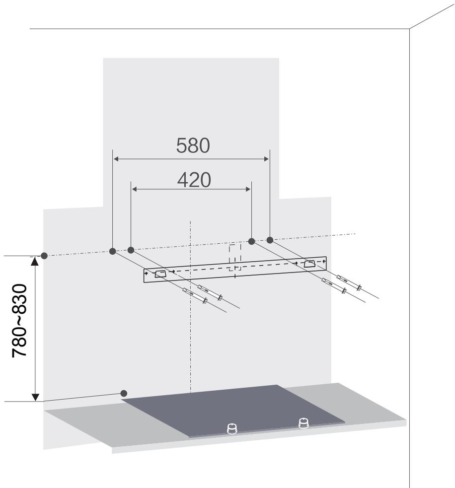
After hang the hood on the installation plate, fasten two screws M5X50, avoid the hood slide off accidentally.
