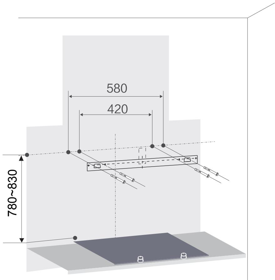
After hang the hood on the installation plate, fasten two screws M5X50, avoid the hood slide off accidentally.
