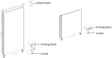
6) Install the refrigerate door on the lower hinge and then install the middle hinge and hole caps.
