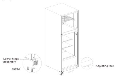
5)Dismantle the limiting blocks and screws on the lower cover of both refrigerator door and freezing door, install them on the other side of both doors; then install the sleeve pipe on the upper cover of the refrigerate door on the other side.
