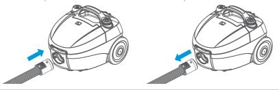
02 Connect the plastic tube to the curves end of the hose.
