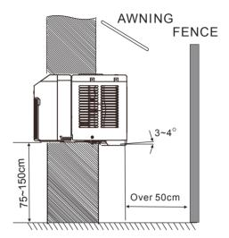
Note: Unit may be supported by a solid frame from below or by a hanger from a solid overhead support.
