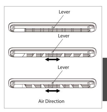
The louvers will allow you to direct the airflow Up or Down(on some models) and Left or Right throughout the room as needed. Pivot horizontal louvers until the desired Up/Down direction is obtained. Move the Lever(s) from side to side until the desired Left/Right direction is obtained.
