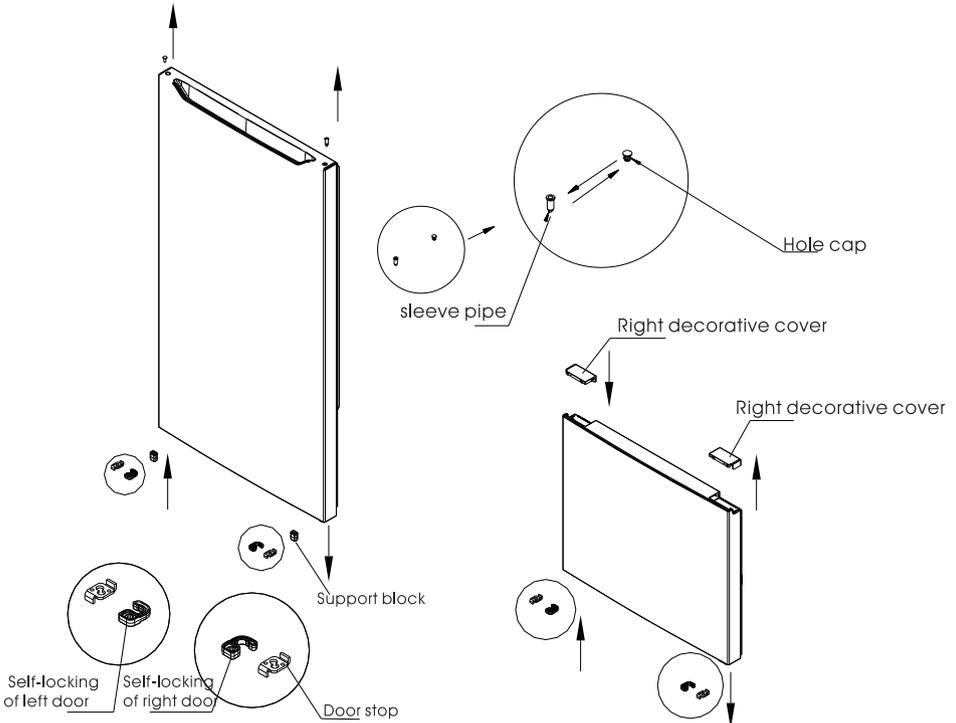
6) Install the door of refrigerator chamber on the lower hinge, the middle hinge on the left side of the refrigerator and tighten the screws, and place the shaft sleeve well. Install the plug pin in the hole on the middle beam at the other end.
