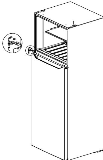
7) Install the door of freezer on the middle hinge, take out the left upper hinge and the cover for the left upper hinge from the accessory bag, install the left hinge and tighten the screws, install the cover for the left upper hinge and tighten the screw, install the right sensor in the original left hole cover, and then fix the hole cover on the right box.
