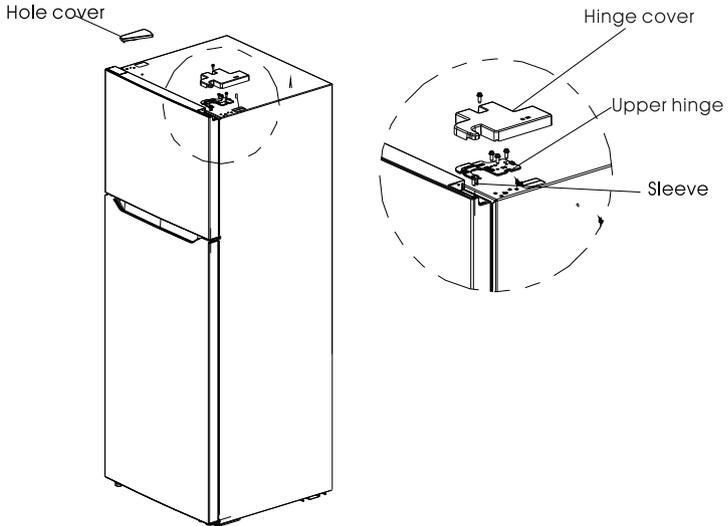
3) Unscrew the hinge screw, take off the middle hinge and the upper shaft sleeve, depart the two hinge hole covers (plug pins) on the middle hinge, and take out the door body of the refrigerator chamber upward.
