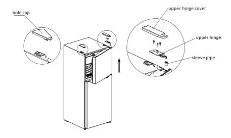
3)Remove the hole caps, fitting screws of middle hinge and middle hinge, then uplift the refrigerator door until it is separated from cabinet completely.
