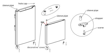
6) Install the Refrigerator compartment door on the lower hinge and then install the middle hinge andhole caps.
