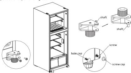
5)Dismantle the right stoppers, sleeve pipes of both refrigerator door and freezer door, and take out the spare left stoppers, install them together with sleeve pipes on left side of both doors; exchange the installation position of sleeve pipe and hole cap on upper end cap of refrigerator door; remove the left decorative cover of freezer door, and move the sleeve pipe from right side to left side.
