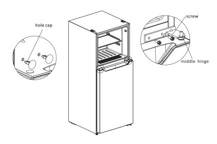
4)Remove the lower hinge assembly from lower right corner and remove the hole cap, screw cap from lower left corner; Dismantle the hinge shaft and adjustable foot and install them on other side of lower hinge; then install the lower hinge assembly on lower left corner by fitting screws, and install the hole cap and screw cap on lower right corner.
