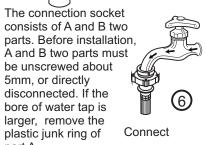
Tightly screw another end of water inlet hose on water inlet valve. (with rubber Note: When tightening the clamping nut, evenly apply the force and do not twist
