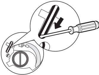
3. Pull down the emergency door pull cord (refer to direction of the arrow in the picture). If unlocked successfully, you will find the door lock icon will go out.
