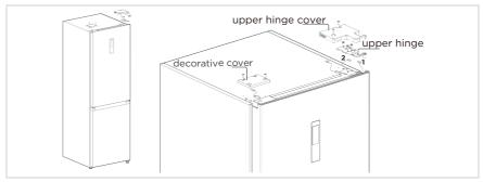
3. Remove the refrigerated door body (be careful not to lose small parts such as the shaft sleeve and stop on the door); Remove the middle hinge and remove the decorative cover of hinge hole on the other side.
