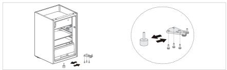
4. Put the door on bottom hinge and assemble the upper hinge, screws, and upper cover.
