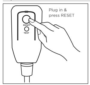
Do not, under any circumstances, cut, remove or bypass the grounding prong.
