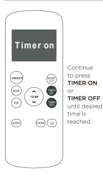
3. Wait 2 seconds, then the TIMER OFF function will be activated. The digital display on your remote control will then return to the temperature display.
