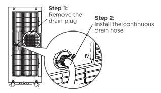
During dehumidifying mode, remove the drain plug from the back of the unit, install the drain connector (5/8" universal female mender) with 3/4" hose.
