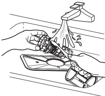
5. Reassemble the filters in the reverse order of the disassembly, replace the filter insert, and rotate clockwise to the close arrow.
