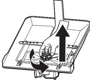
2. Rotate the filter insert counterclockwise to unfasten and then detach the filter insert.
