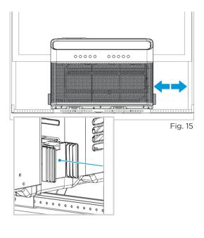
B. Apply Window Sealing Foam to the Side Arm Foam as shown. Note that the Window Sealing Foam attaches to the side next to the air conditioner.
