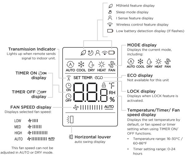
This display is blank when operating in FAN mode.
