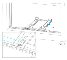
D. Check the level again and ensure the bracket feels secure. After making any necessary adjustments, insert the cotter pins into the Main Support Pins.
