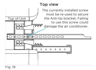
The image shows how the Anti-Tip Bracket is to be installed in the window track. Note the Side Arm Foam was removed for illustration purposes only.
