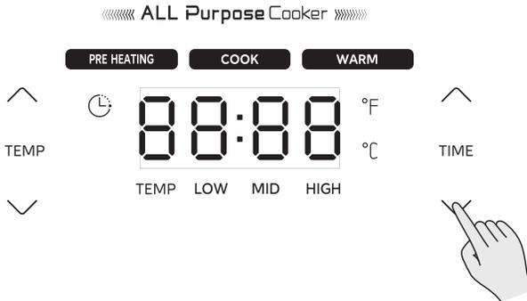
4. Press the temperature adjustment button “∨” or “∧” to set the cooking temperature. (except “STEAM” function)
