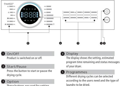
These buttons are used for setting additional functions.
