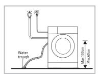
2. Connect it to the branch drain pipe of the trough.
